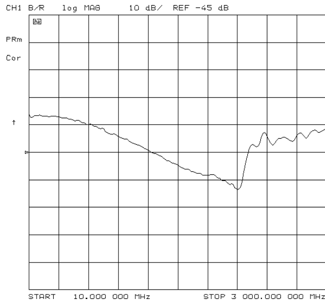
Figure 2-35 Example Mixer LO to RF Isolation Measurement
